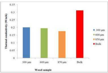
Figure 2: Thermal conductivity as a function of wood sample for *Milicia excelsa* (Iroko).
