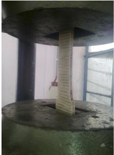
Fig.3.1 Laminate before Tensile Test
