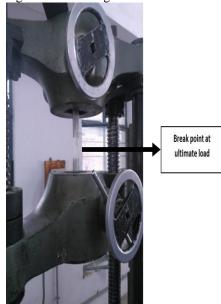
Fig.3.2 Laminate during Tensile Test
