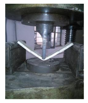
Fig.3.3 Laminate before Bending Test
