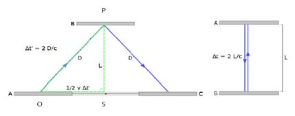
Fig. 5 Moving light clock and Velocity Time Dilation Theory.
