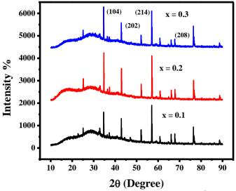
Fig. 3 The XRD of LSC sintered at 1000°C
