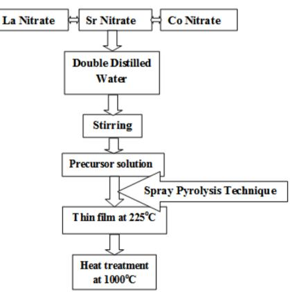
**Fig. 2** Flow chart of spray deposition technique
