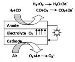
Fig. 1 Solid Oxide Fuel Cell
