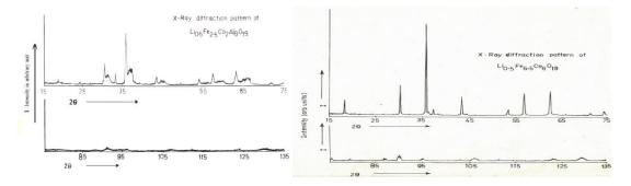
Fig.-1. XRD Diffraction of compound Li<sub>0.5</sub>Fe<sub>2.5</sub>Al<sub>8</sub>Co<sub>2</sub>O<sub>19</sub> and compound Li<sub>0.5</sub>Fe<sub>6.5</sub>Co<sub>6</sub>O<sub>19</sub>
