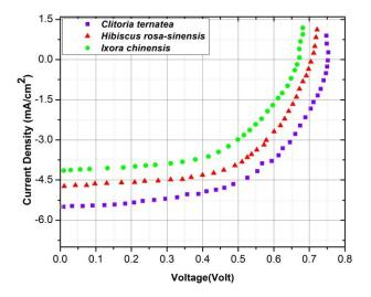
Fig. 5a. Current density (J) - Voltage (V) characteristics of DSSCs.
