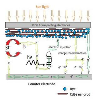
Fig. 1 The schematic diagram of fabricated DSSC.
