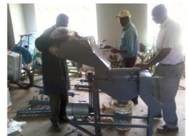
Fig 4: Threshing operation using the prototype thresher
