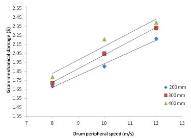
Fig. 6 Grain damage versus peripheral drum speed at different levels of drum diameter
