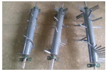
Fig. 3: Threshing drums of different diameters
