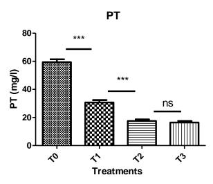
Figure 2: Average values of total phosphorus. The horizontal bars represent the standard error during the process. \*\*\* p <0.0001; ns: not significant. (Bonferroni test)
