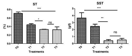
**Figure 1**: Concentration of Total Solids (ST) and Total Suspended Solids (TSS) in%. The horizontal bars represent the standard error during the experiment. \*\*\* p <0.0001; \*\* p <0.05; ns: not significant. (Bonferroni test) treatments
