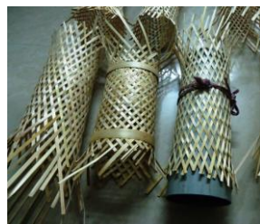
Conversion of Matt to cylinder using standard fixture
