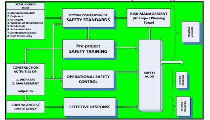
Figure 3: Integrated Proactive Control and Reactive (PCR) Safety Model For Typical Construction Company
