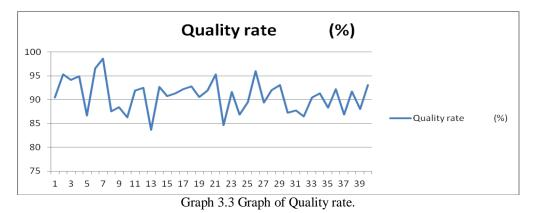
Above graph 3.3 will represents the Quality rate of L.G industry for 40 shifts. Here we can observe that similar to Availability and Performance rate, quality rate is also not showing constant values. It's fluctuating in Zigzag manner and varies continuously from standard value of 99.9%.
