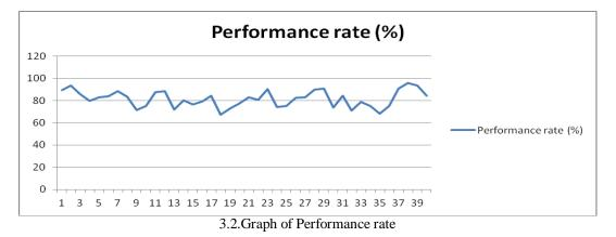
Above graph 3.2 represents the 40 shifts values for Machine performance rate of L.G industry. Mainly it gives the speed losses from standard value. From graph we can observe that performance rate also continuously fluctuating from its standard value of 95%. For every 2 to 3 shifts we can observe change in direction of performance rate line.
