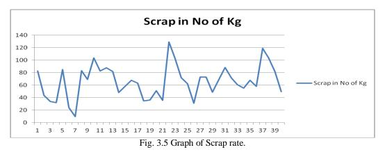
Above graph 3.5 represents the scrap rate of L.G industry. Reason for scraps can be categorized in to two category and they are: 1. Trail run scrap and 2.Production defects. Here we can observe that whenever continuous production of same type of pipe takes place, scrap rate will be decreased and whenever changeover is there we can observe increase in scrap. Hence this variation is mainly due to trail run scrap.
