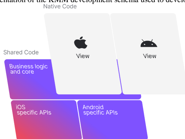
Figure 2: Representation of the KMM development schema used to develop the APP +Leite. 8
