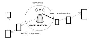
Fig.1. . In a adhoc network the mobile nodes can form coalitions to help forward data from a base station to other mobile nodes which are out of the transmission variety of the base station.
