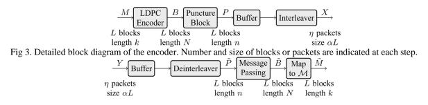
Fig 4. Detailed block diagram of Bob's decoder. Number and size of blocks or packets are indicated at each step.
