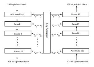
AES Encryption AES Decryption Fig. 5. AES Block Diagram
