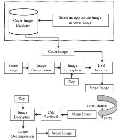
Fig 2. Block diagram of Proposed Steganographic system
