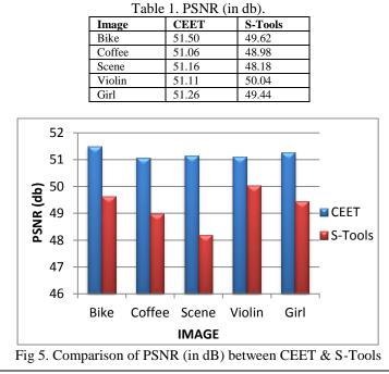
High PSNR indicates good perceptual quality of stego-image. Here the resultant PSNR value of CEET is better than that of S-Tools. Table 2 represents the correlation coefficient for cover image and stego image. Correlation coefficient is very high which indicates the cover image and stego image are highly related.
