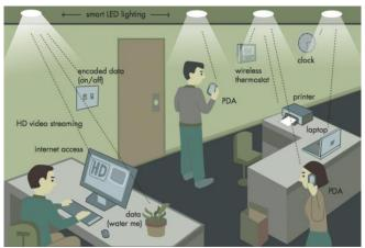
Fig. 1: Devices accessing internet through LED
