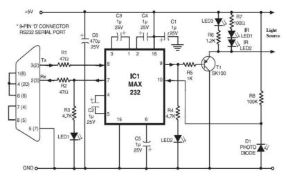
Fig.2: Circuit Diagram for driving LED and photo-diode
