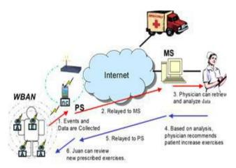
If we come into the detail of how the data is given to the PS in which form it is as follows .Firstly the network coordinator(NC) acts as interface between the person and the PS helps in using the data communication standards sensor nodes get initial commands and give response to the queries from PS. The nodes collect raw data continuously and send processed data to the PS.
