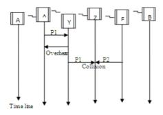
Fig. 4 Receiver collisions in MANETs
