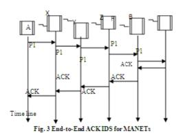
In fact, many of the existing IDSs in MANETs adopt an acknowledgment-based scheme, including TWOACK and AACK. The functions of such detection schemes depend on the ACK packets. Hence, it is crucial to guarantee that the acknowledgment packets are valid and authentic. To address this concern, a digital signature is adopted in recent secure IDS named Enhanced AACK (EAACK).
