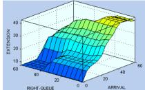
Figure 19: Input variables Arrival, Right-Queue Vs output variable Extension
