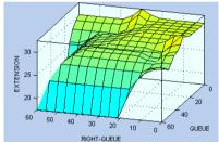
Figure 20: Input variables Queue, Right-Queue Vs output variable Extension
