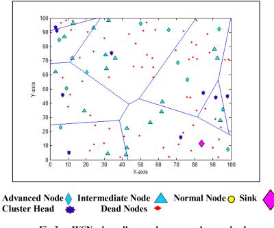
Fig.3 WSN when all normal sensor nodes are dead
