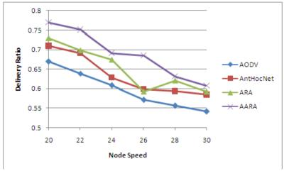
Figure 7.7: Delivery Ratio Vs Node Speed.
