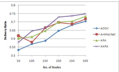
Figure 7.1: Delivery ratio Vs node density
