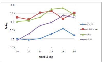
Figure 7.8: End-to-End Delay Vs Node Speed.
