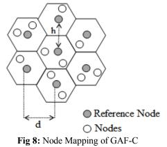
The horizontal distance between two reference nodes is h and the vertical distance between the two is d. Each cell has one active node used for routing the data and other nodes are in sleep state.
