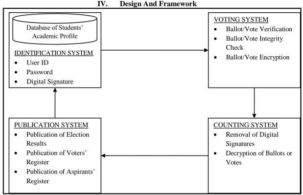
Figure 2: Simplified System Architecture of the Secure Intranet Voting System (SIVS)
