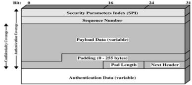
Figure 5: Encapsulating Security Payload
