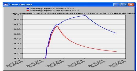
Figure 12: Core Router time average (in processor Forwarding memory queue size (incoming packets)
