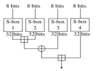
Fig 3: Blowfish Cryptographic Algorithm
