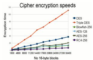
Fig4 Comparison of encryption times for various common symmetric encryption algorithms
