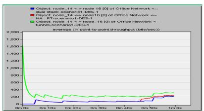
Fig. 5 Throughput performance of Dual-stack, NAT-PT, and Tunneling configurations.
