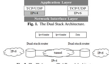
Fig. 2. The IPv6 over an IPv4 Tunnel Architecture
