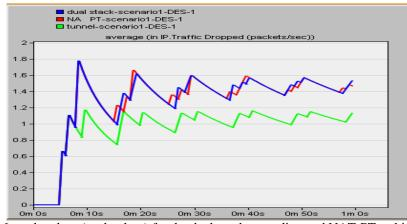
Fig. 6 packet drop (packet loss) for the dual-stack, tunneling and NAT-PT techinques.
