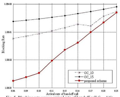
Fig. 5. Blocking rate versus arrival rate of handoff call ( $\lambda_n = 1/6$ ). Fig. 6 presents the throughput versus inter-arrival time of handoff calls for GC\_10, GC\_15, and proposed schemes. The throughput decrease with the inter-arrival time of handoff calls. This is
