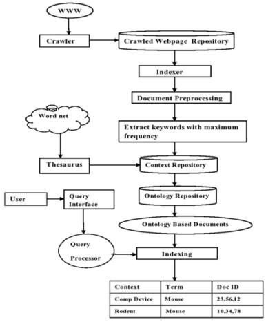
Fig1: Architecture of context based indexing
