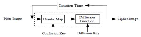
Figure 2. The chaos-based image encryption scheme. Here, the plain-image is encrypted into cipher-image through chaotic confusion, diffusion, and repeated iteration.
