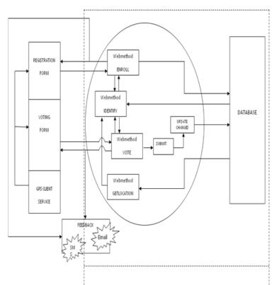
Figure 2: Model of the Developed E-voting System.
