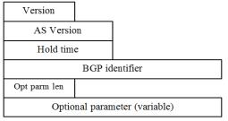
Fig 2: OPEN message format(Source: RFC 4271)
