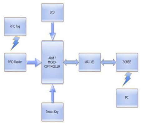
Fig 4.2: Block Diagram Of System At Trolley
