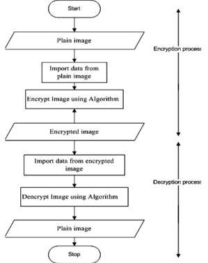
Figure 2: The flow chart diagram for the encryption and decryption process.
