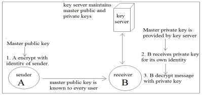
Fig.1 Process of Identity Based Encryption (IBE)
