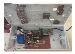
Plate 3. The output/ keypad unit design (the inside view)
