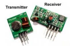
Figure 6. Radio-Frequency (RF) Link: Transmitter/Receiver modules
