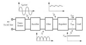
Figure 2.Complete Block diagram of power supply
