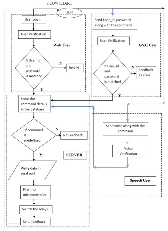
Figure 3.2 Proposed flow-diagram
