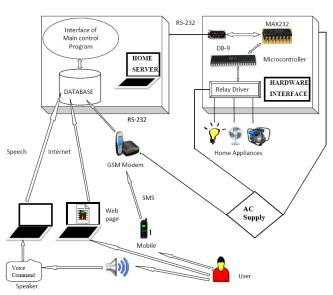
Figure 3.1: Block Diagram of overall proposed system
