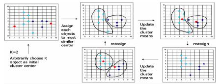
Fig2. Working of K- means algorithm.
