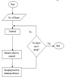
Fig1. Flowchart of K-means
