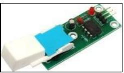
Fig.6 (Accident Sensor)
