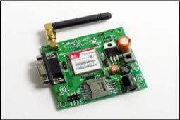
Fig.7 (GSM Modem)
