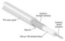
Figure 10. Tight Buffer CableStructure
