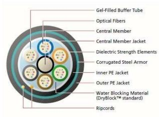
Figure 4. Fiber optic cable
