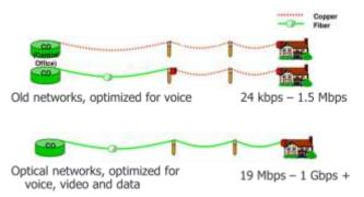
Figure 12. Comparing FTTH and copper network
