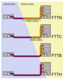
Figure 13. Fiber To The x (FTTx)
