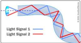
Figure 2. Signal transferring inside fiber
