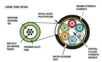
Figure 7. Cross-section of loose tube cable
