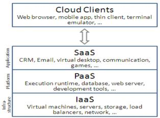
Figure1: Cloud Computing Architecture
