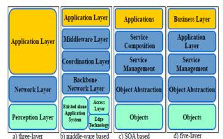
Figure 2: IOT Layered Architecture
