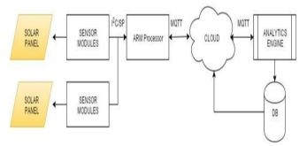
Figure 1: Data Acquisition Architecture
