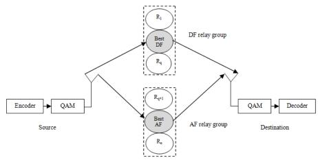
Fig. 1: The proposed Hybrid Relay Selection.
