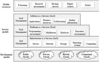
Fig3. Cloud Computing Structure For University [15]
