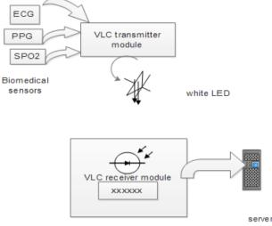
Fig2. Experimental setup for indoor VLC system
