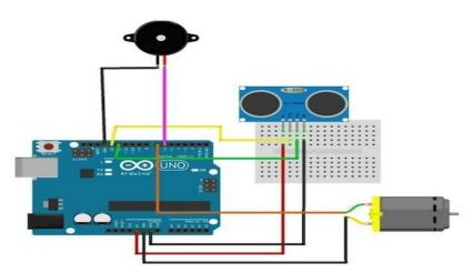
Figure 5: Arduino connections
