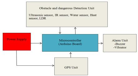
Figure1: Proposed system design of the smart stick.
