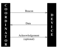
Fig.2 Communication to a coordinator in a beacon enabled network
