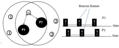
Fig.4 Indirect beacon frame collision
