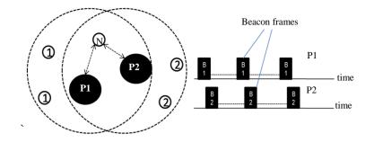
Fig.3 Direct beacon frame collision
