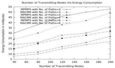
Fig.9: Number of Transmitting Nodes vs. Energy Consumption in millijoules
