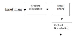
36-D HOG Feature Extraction Figure 2: Block Diagram for extracting HOG from an input image
